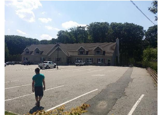
A bioretention system can be implemented in the grass area between the entrance of the parking lot and the building to capture, treat, and infiltrate stormwater runoff from the driveway. A preliminary soil assessment suggests that the soils have suitable drainage characteristics for green infrastructure.
