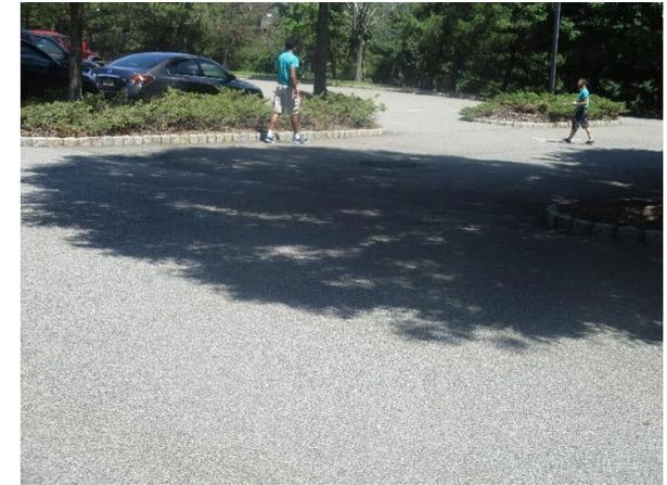
A large amount of runoff is generated by the parking lot during storm events. Two large sections of parking spaces can be replaced with pervious pavement to manage the majority of this runoff. A preliminary soil assessment suggests that more soil testing would be required before determining the soil's suitability for green infrastructure.
