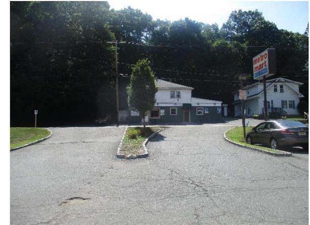
A large amount of runoff is generated by the parking lot during storm events. The parking spaces closest to the building can be replaced with pervious pavement to allow water to infiltrate through the surface. A preliminary soil assessment suggests that the soils have suitable drainage characteristics for green infrastructure.
